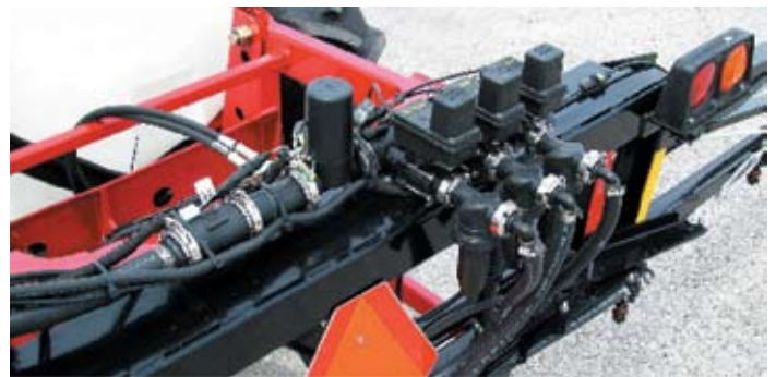
Sealed on/off valves are located on the boom center section for quick response.
